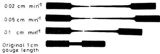
Figure 2 Fractured tensile specimens of the boron-free steel (K1970) strained at various rates at 900°C.
